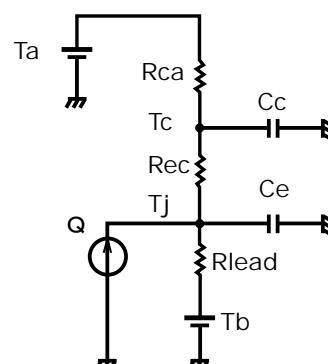
T<sub>j</sub>: Element temp. C<sub>e</sub>: Element heat capacitance R<sub>ca</sub>: R<sub>th</sub> (Surface to amb.)
