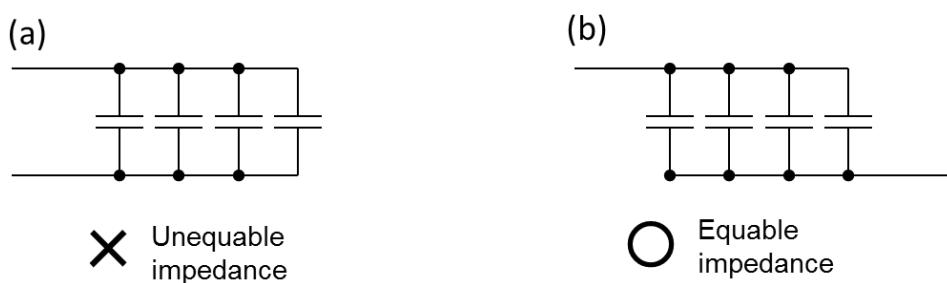
Fig. 28 Wiring for parallel connection of capacitors
