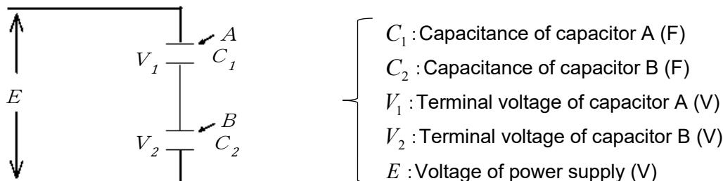
Fig. 26 Series capacitor connection
