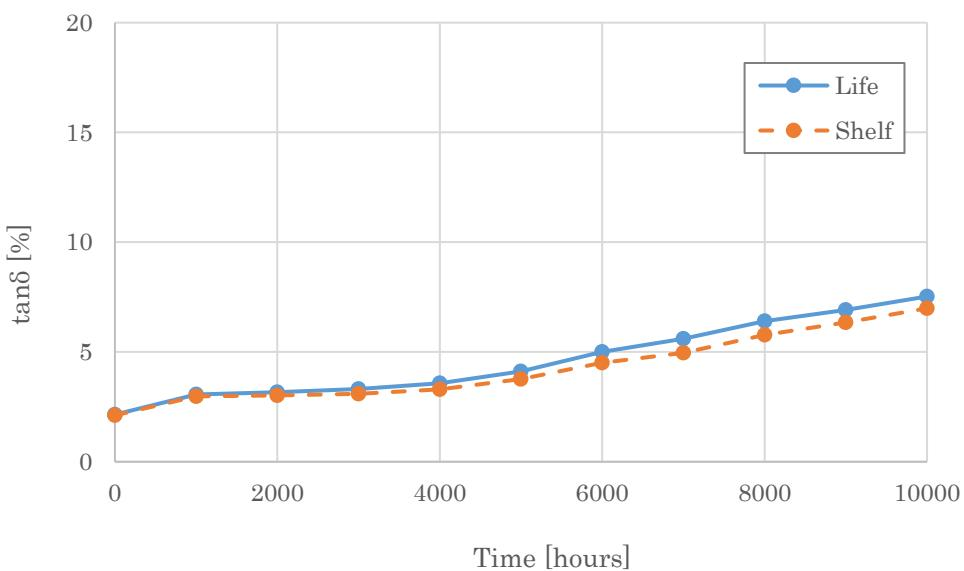
Fig. 19 Changes in tangent of loss angle ( $\tan \delta$ ) with time at 105 °C
