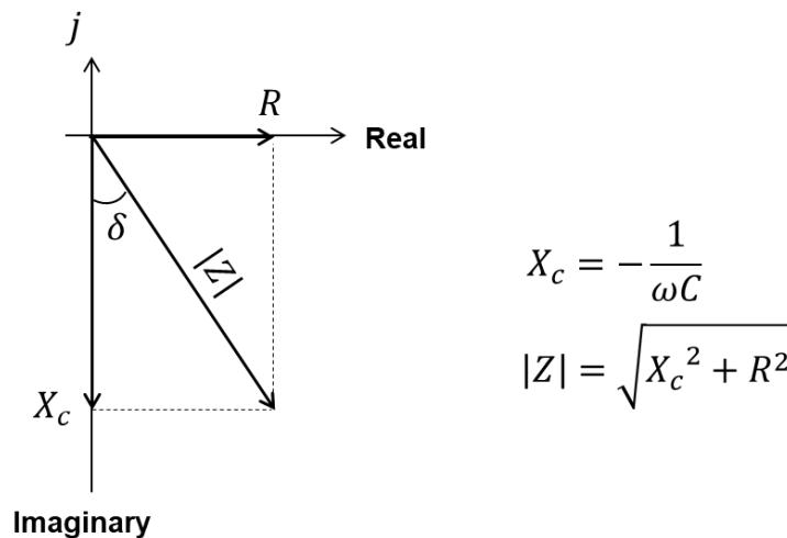
Fig. 9 Impedance and Loss angle of Capacitor
