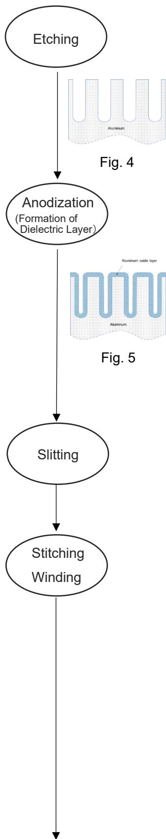
To obtain higher capacitance, surface area of aluminum foil for electrolytic capacitor increases through the etching process.
