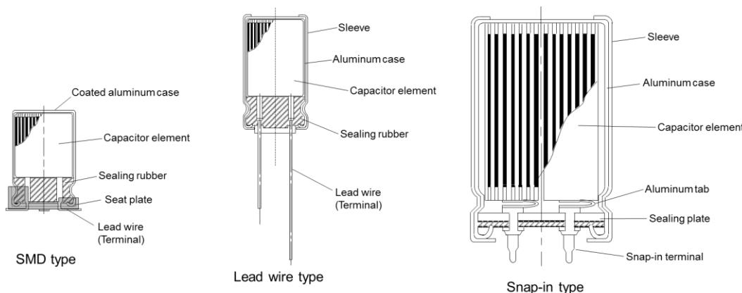
Fig. 3 Basic structure of aluminum electrolytic capacitor
