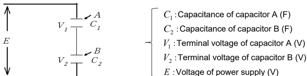
Fig. 26 Series capacitor connection
