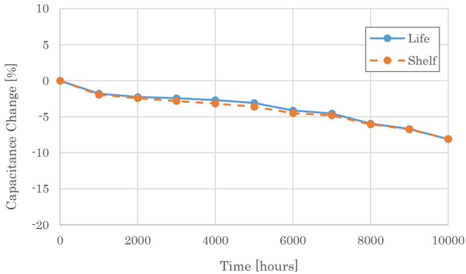
Fig. 18 Changes in capacitance with time at 105 °C
