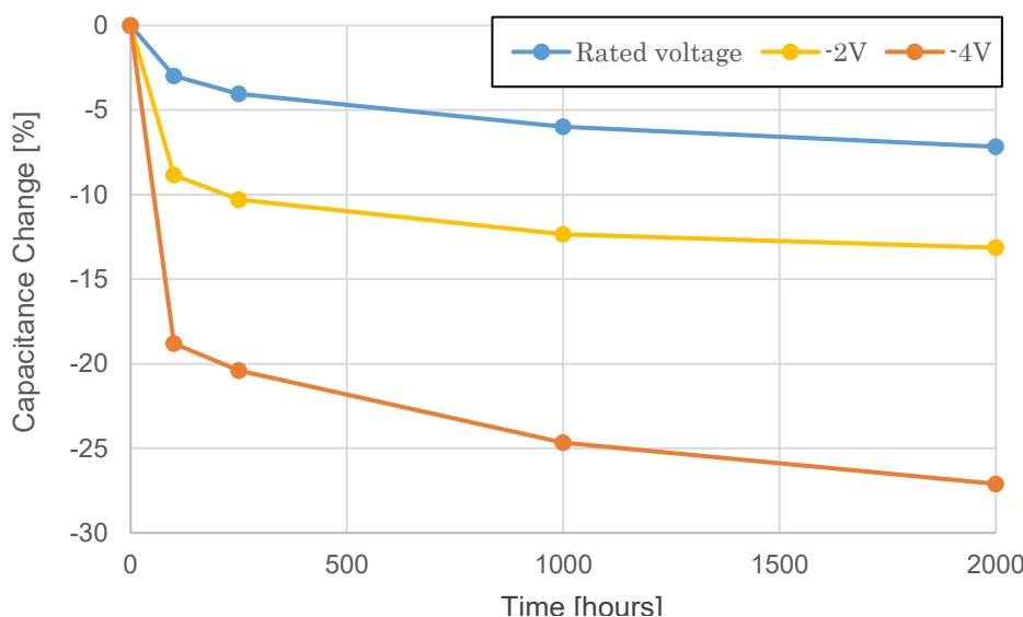
Fig. 25 Capacitance change when reverse voltage is applied
