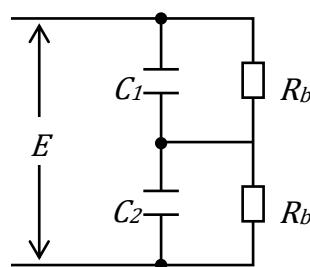
Fig. 27 Series capacitor connection with balance resistance
