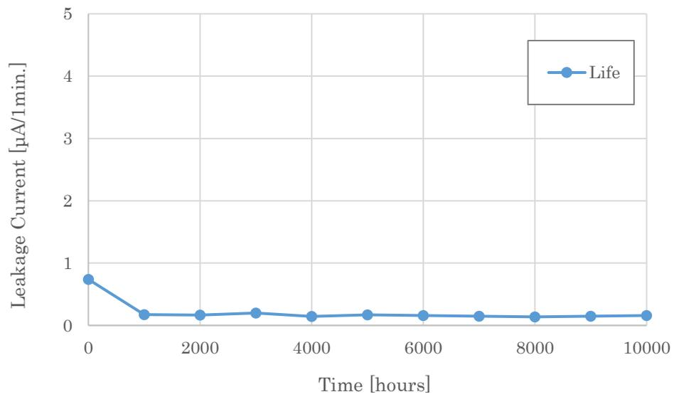
Fig. 20 Changes in leakage current with time at 105 °C (only life)
