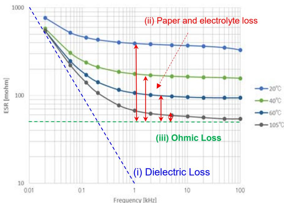
Fig. 11 ESR Characteristics of Aluminum Electrolytic Capacitor
