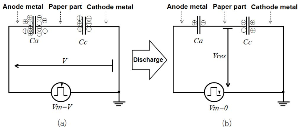
Fig. 23 The charge transformation on charge and discharge
