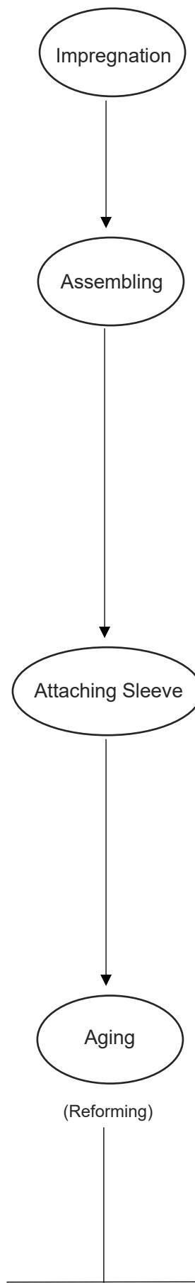
The wound element is immersed into an electrolyte bath under either a low or normal air pressure condition to impregnate the paper. Electrolyte contains one or more polyhydric alcohols such as ethylene glycol as the major solvent and one or more ammonium salts as solutes to restore the damaged dielectric layer and significantly improve the performance and life of the capacitor.
