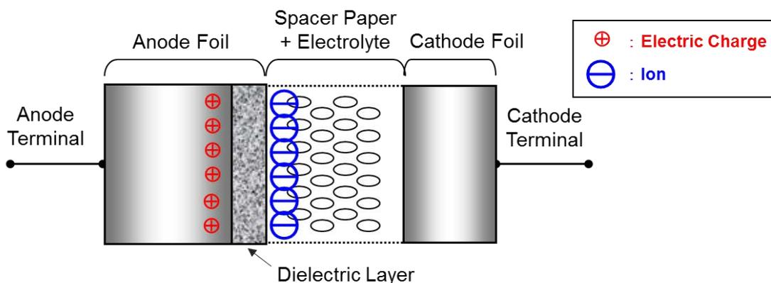
Fig. 1 Basic construction of an aluminum electrolytic capacitor
