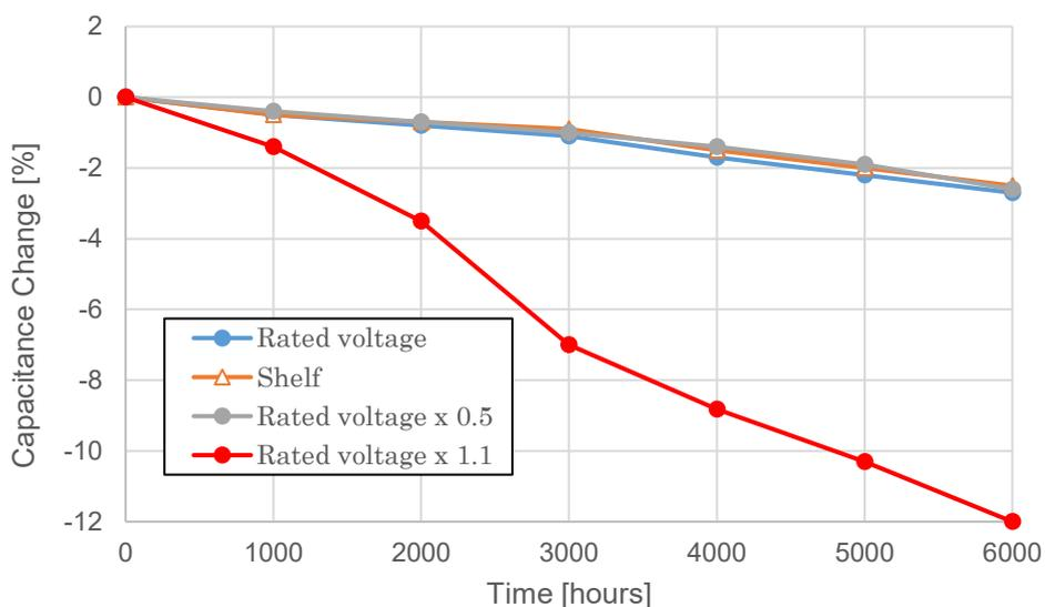
Fig. 24 Capacitance change when overvoltage is applied
