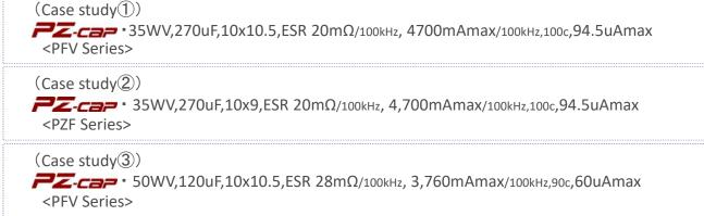
In addition, further Size reduction is possible by optimizing the thermal design. Please consult us about capacitor's thermal model & thermal simulation.
