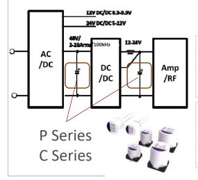
(Case study 1) DC/DC input: Replacement of ceramics capacitor MLCC •100WV,2.2uF, Number of capacitor 3 to 4pcs •80WV,22uF,8x10.5,ESR 35mΩ/100kHz,-40c, 2,580mAmax/100kHz,100c <PFV Series>
