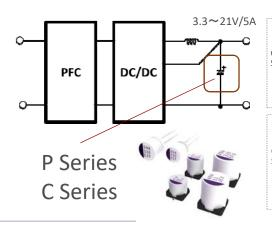
(Case study 1) Replacement of conductive polymer solid capacitor
