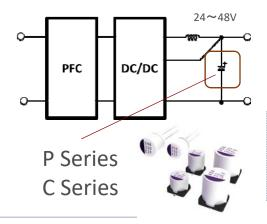
(Case study 1) DC/DC 24V Output -2-cap ·35WV,270uF,10x9,ESR 20mΩ/100kHz,-40c, 4,550mAmax/100kHz,100c <PZE Series>
