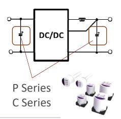
(Case study(1)) Replacement of ceramics capacitor (MLCC) MLCC ···50WV,4.7uF,2012 Number of capacitors 4pcs **PZ-cap** •50WV,22uF,6.3x6.1 Number of capacitor 1pcs <PFV Series>
