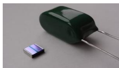
Photo. 2 Size comparison example with film capacitor (10 \mu\text{F} item)
